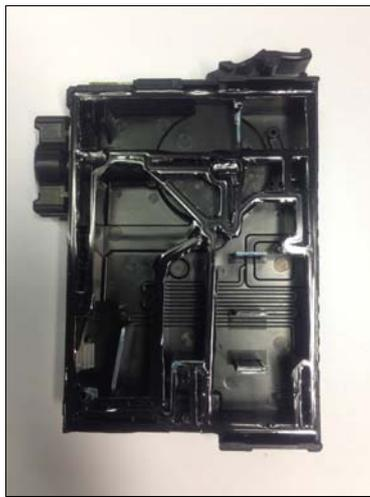
Epson cyan cartridge pre-flushed and flushed.
