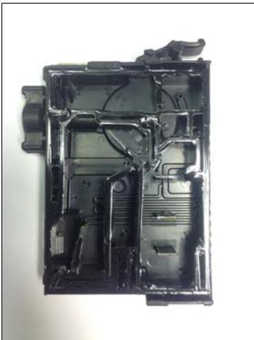
Epson yellow cartridge pre-flushed and flushed.
